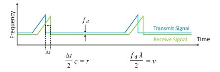
Figure 3. FMCW range (r) and velocity (v) signals
