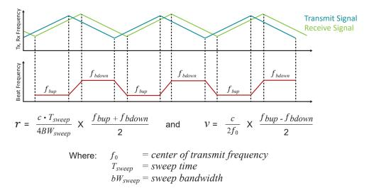
Figure 4. Triangle Wave FMCW modulation
