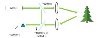
Figure 2. Graphic description of a coherent detection LIDAR system
